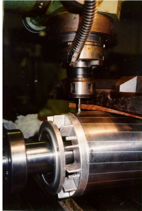
Figure 7: For broken one rotor bar a hole is drilled into the aluminum part of the squirrel cage rotor
