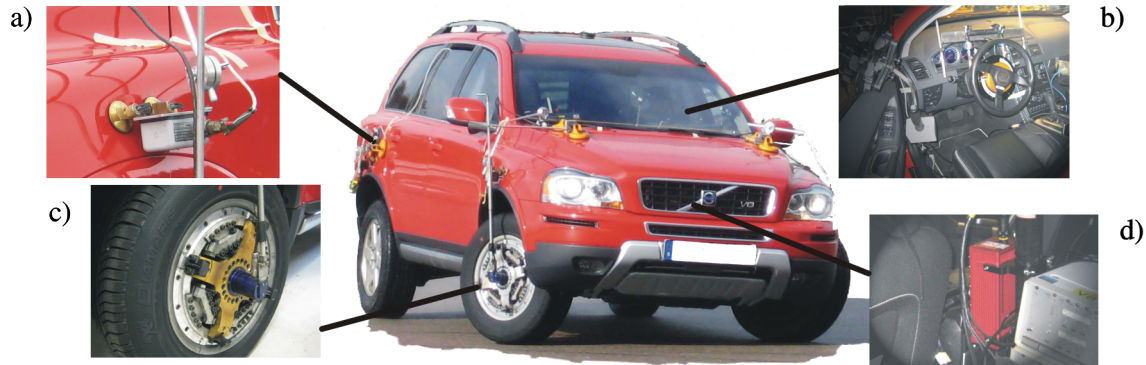
Figure 6: The tested vehicle equipped with a) wheel travel sensors, b) steering robot, c) measuring wheels and d) gyro platform
