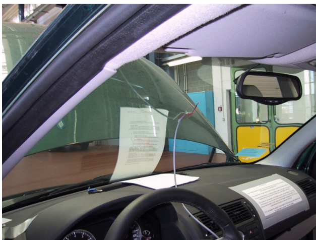
Fig. 10 Thermocouple attached to the inner surface of the windscreen
